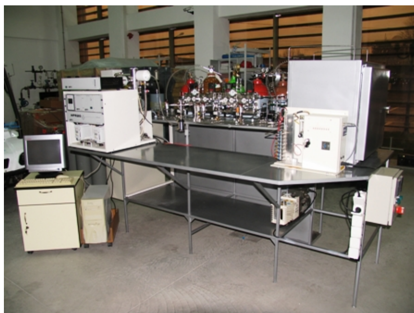
Instalatia experimentală SSITKA - Steady State Isotopic Transient Kinetic Analysis
