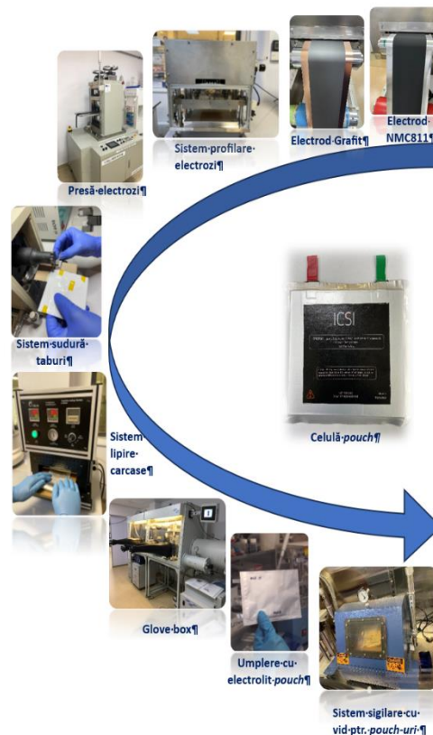
Technological flow for producing pouch cells based on NMC811/Graphite
